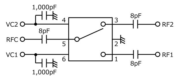
The application circuits and their parameters are for reference only and are not intended for use in actual designs. DC Blocking Capacitors are required at all RF ports.
