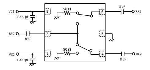
The application circuits and their parameters are for reference only and are not intended for use in actual designs. DC Blocking Capacitors are required at all RF ports.
