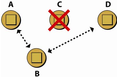
ZigBee is an internationally recognized open protocol, based on IEEE's 802.15.4 standard. It's backed by the ZigBee Alliance, which ensures interoperability and compatibility of components from a wide choice of suppliers. ZigBee operates in the 2.4 GHz ISM (industrial, scientific, and medical) band. ISM band frequencies have been set aside for unlicensed operation, meaning anyone is allowed to use them without having to obtain a license from a governmental regulatory body, for example the FCC.
