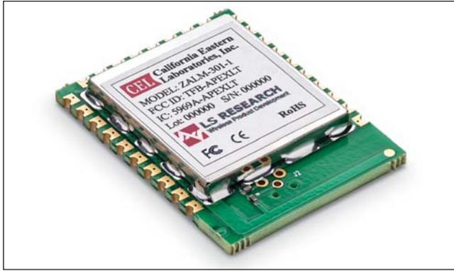
Figure 1 · A variety of ZigBee/802.15.4 transceiver ICs are available. Ember™ combines an RF transceiver with a flash-based co-processor in its EM260 chip. The EM260 stores the ZigBee stack in its flash memory, but takes commands from the processor that is resident in the end-user system. CEL's Apex LT combines the EM260 with a 100 mW power amplifier in an easy-to-use, drop-in radio module. FCC, IC and CE certified, these modules are ideal for designers looking for fast time-to-market.
