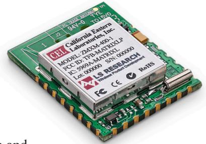
Designed for low cost, low power networks, Matrix modules are ideal for home and building automation, industrial control, security, and remote sensor applications. Output power can be configured up to 10mW, enabling performance to be optimized for specific applications. Since they're limited to 10mW, Matrix modules are ideal for regions where regulatory agencies limit transmission power.
