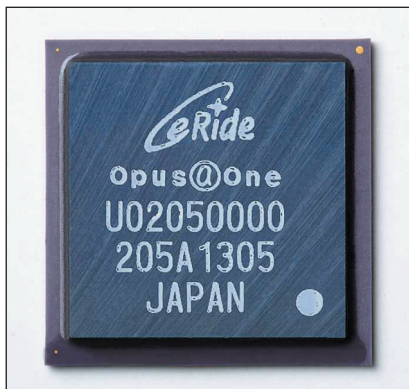
2. The Opus One baseband IC combines state machines, peripheral devices, and a low-frequency clock in a 10 \times 10 -mm ball-grid-array (BGA) package.
