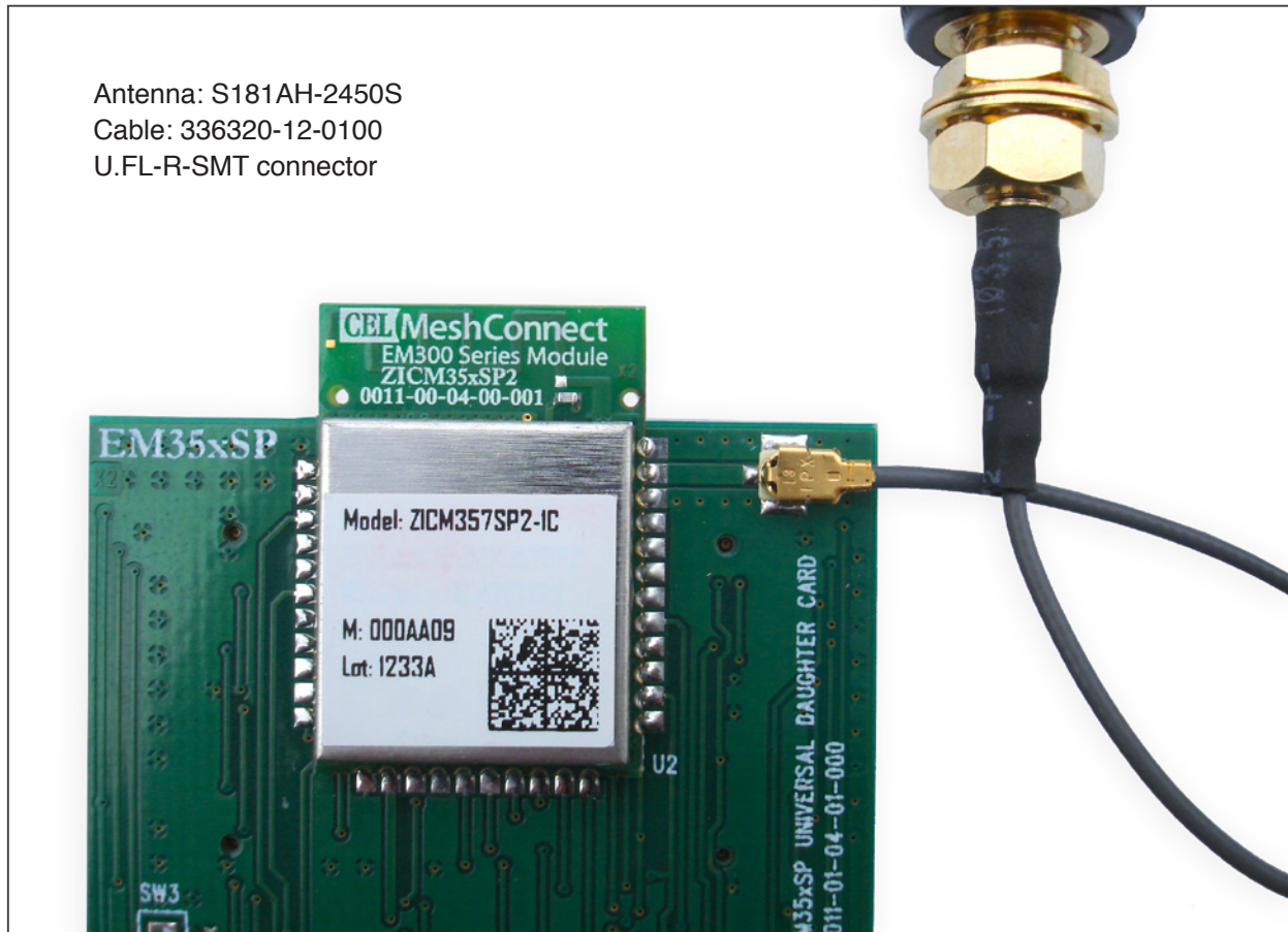
Figure 4. Implementation using connector, cable and external antenna
